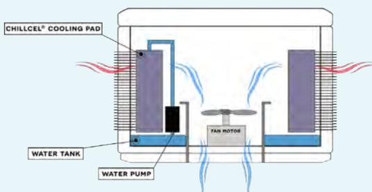
Evaporative cooling is often installed for comfort cooling reasons, to improve working conditions inside a manufacturing plant or a warehouse, for example.
